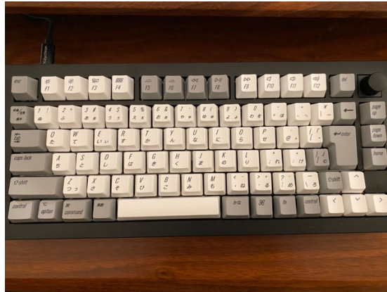
Example of a JIS layout mechanical keyboard (Keychron Q1), which is close to the Apple Japanese Keyboard Layout.
